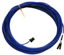
E0070 Electrical harness for 7-way power 70' cable with terminals mounted: Delphi connector at low-pressure sensor and female .180 bullet connectors at low-pressure warning light (customer to cut and splice at connection to trailer 7-way power)
