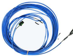
E5555 Electrical harness for 7-way power Pre-assembled harness for connection to trailer 7-way power, terminals mounted: Delphi connector at low-pressure sensor, female .180 bullet connectors at low-pressure warning light, bare copper at trailer 7-way power, no cutting/splicing * 5' length from 7-pole power connection to junction, 5' length from warning light to junction, 55' length from junction to low-pressure sensor
