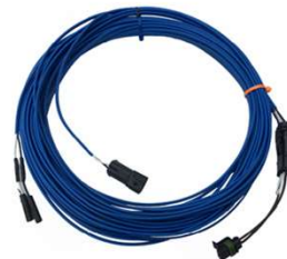
E2166S Electrical harness for ABS power Pre-assembled harness for connection to trailer ABS power, terminals mounted: Delphi connector at low-pressure sensor, female .180 bullet connectors at low-pressure warning light, Delphi connector at trailer ABS power, no cutting/splicing * 21' length from low-pressure sensor to ABS power connection, 66' length from low-pressure sensor to warning light
